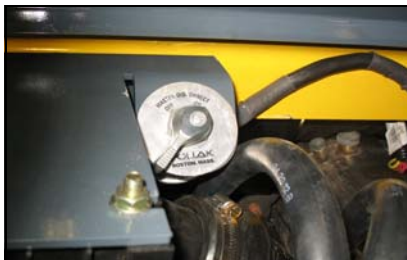
Figure 14 – Battery Disconnect Switch
