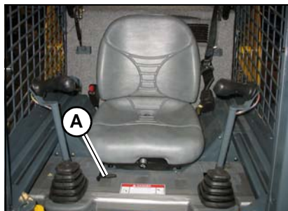
Figure 4 – Operator's Seat Horizontal Adjustment
