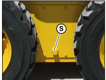
Figure 112 – Chaincase Fill/ Check Plugs
