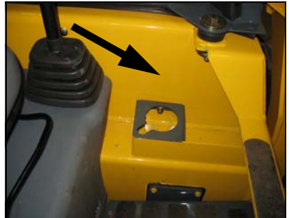
Figure 1 – Fire Extinguisher Location
