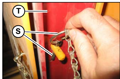
Figure 11 – Lift Arm Support Storage Lynchpin Removal
