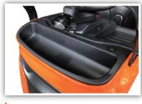
Safety flanks and non-slip surface materials on both sides of Large storage tray can be used for storing
