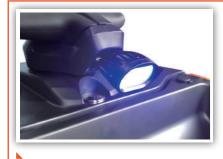
The standard blue light does not only automatically lit while the ruck forwarding but also follows the handle to turn while the truck turns. It greatly improves the safety of the operation.
