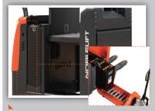
Sideways battery exchange compartment plus adjustable handling bracket makes battery replacement easier and quicker.
