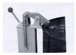
to bite the drum firmly and for the bulbous knob to lock the clamp (Part No.1). Continue to pump up the lifting frame (Part No.2) by handle (Part No.4) and then the drum will be lifted.
