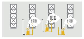
The geoguidance navigation technology works without the need for dedicated infrastructure, enabling it to integrate easily into existing operations. It simply maps the physical features and structures to self-locate and navigate, which means it's quick and easy to modify or create entirely new paths when there are changes to the environment, or to the missions that your robots are required to complete.
