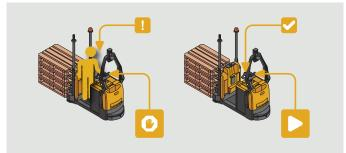
By switching from automatic mode to manual mode at the touch of a button, or movement of the tiller, the robotic lift truck can easily accommodate changing operational needs, giving the operator the opportunity to take control when appropriate and perform other tasks as and when required.
