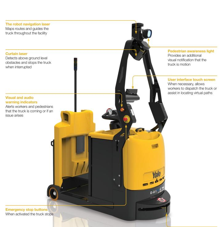
Laser has two fields. Warning and STOP (also called Safety). Breaking the warning field will slow the truck down. Breaking the STOP field will stop the truck. If the obstacle is cleared, the robotic can automatically re-start in all cases for the warning field and some for the
